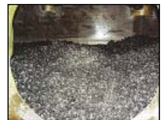
Götaverken Miljö AB's ADIOX system, tower packing material with carbon as an extra dioxin barrier, integrated in the scrubber system.
